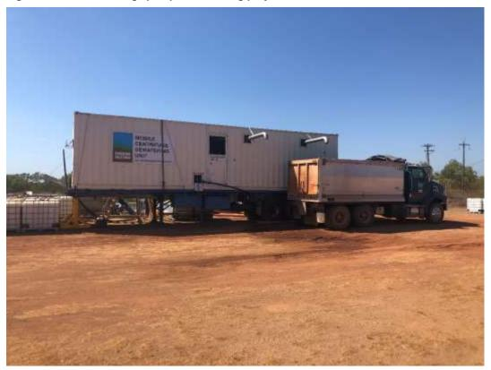
Figure 5: Containerised centrifuge unit (Dredging Solutions).
