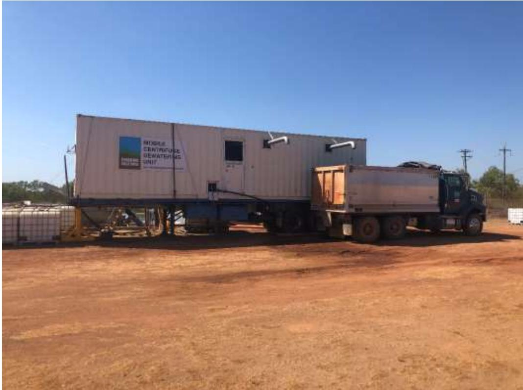
Figure 5: Containerised centrifuge unit (Dredging Solutions).
