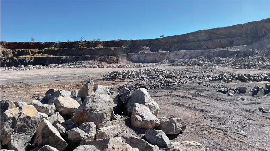
*Figure 6-11: Jubilee Quarry overburden stockpile, currently sorted for rock supply.*
