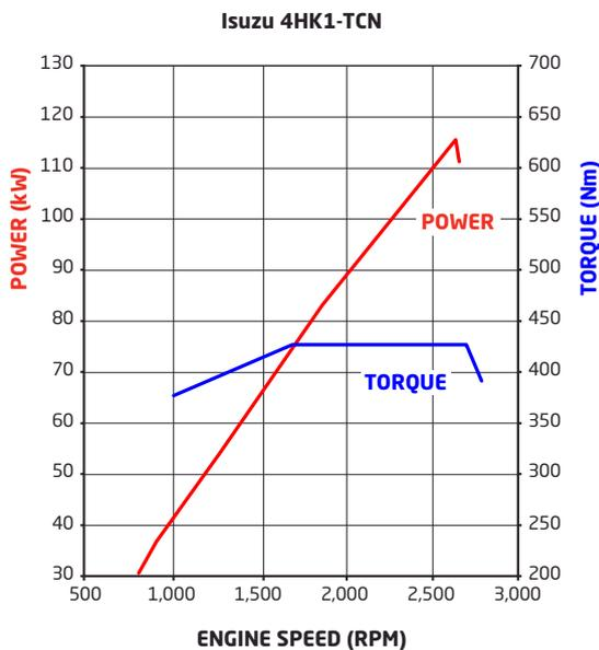
\* Maximum torque electronically limited to 377Nm (DIN) when in low range first or reverse gear
