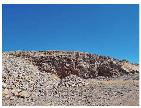
Figure 6-8: Jubilee Quarry current working face - heavily fractured and not suitable for rock armour.
