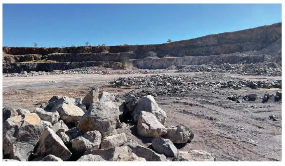
Figure 6-11: Jubilee Quarry overburden stockpile, currently sorted for rock supply.
