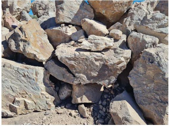
Figure 6-6: Fractures rock in the 1000+mm diameter stockpile.
