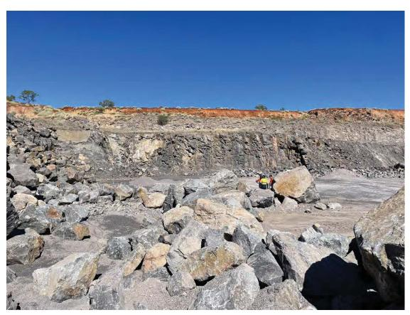
Figure 6-12: Stockpile of oversized rock armour.
