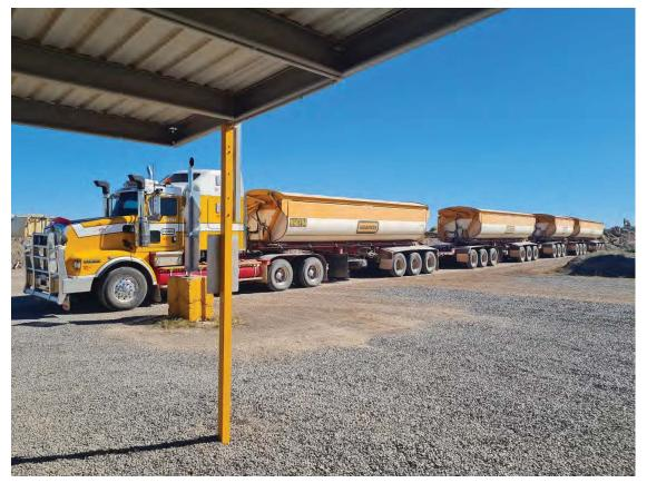
Figure 6-2: Side tipper road train at Cloncurry. Capacity 100t (25t per dog trailer).
