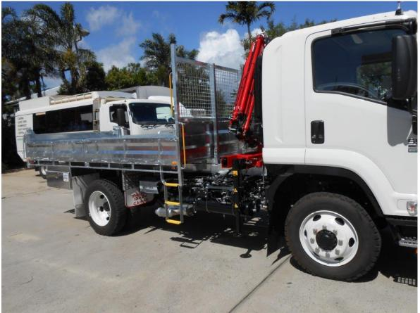
Figure 1 Tray and Crane Example
