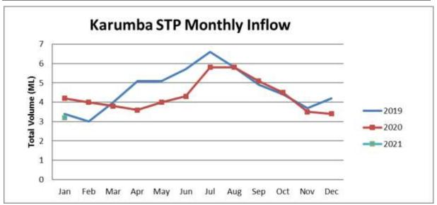
Figure 4: Total Monthly inlet flow for Karumba STP.
