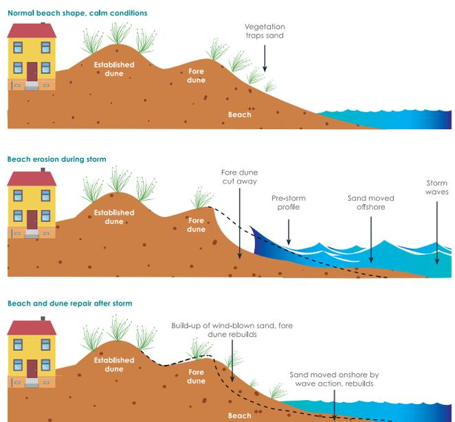
Figure 4. Natural short term erosion and dune rebuilding process
