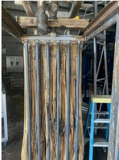
**Photo:** Membrane De-ragging and inspection
